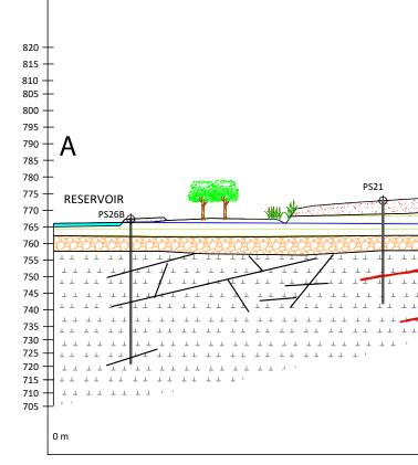
Diagram of the conceptual model of the Sardas landfill
